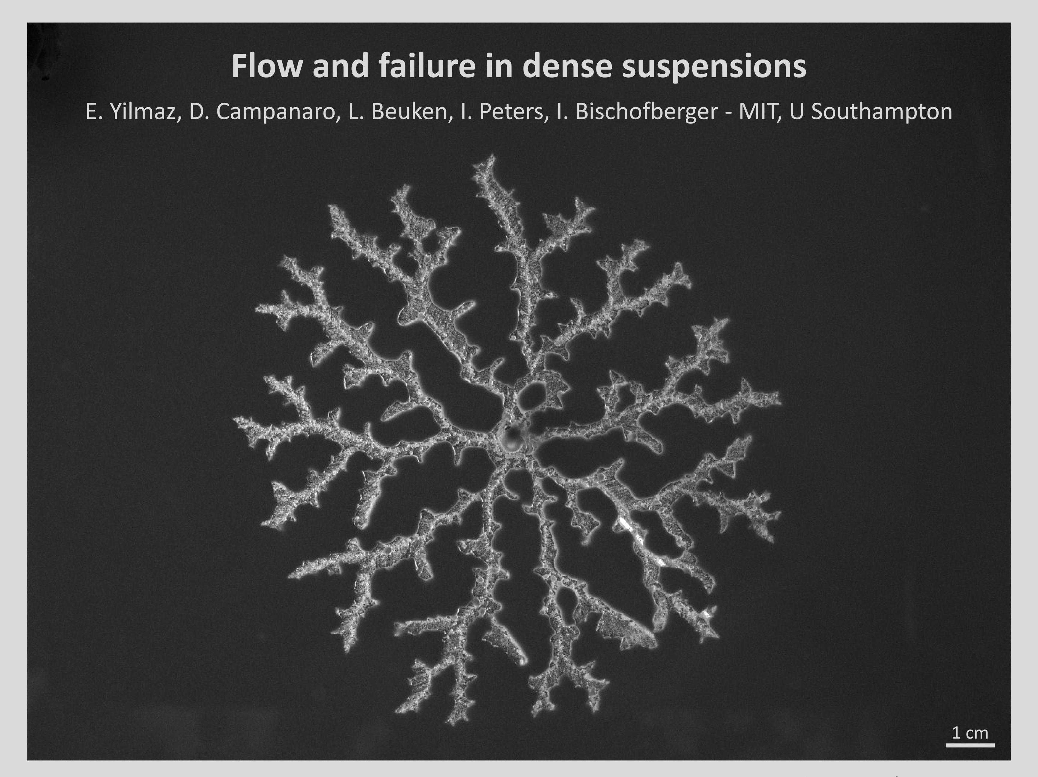
The injection of air at a controlled pressure into a confined 2 mm thick layer of a dense suspension (cornstarch/water mixture at 57.5 wt%) leads to the formation of branched fractures at a gauge pressure P = 10 kPa (top) and the formation of straight fractures at P = 20 kPa (bottom). The transition occurs when the characteristic width of the branched fractures becomes comparable to the thickness of the layer.
